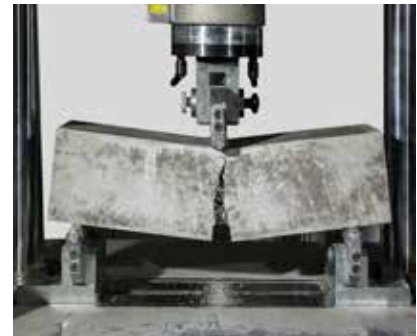
Beam test: EN 14651
